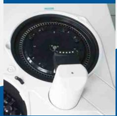
Long-life direct read cuvettes with integrated Cuvette Quality Assurance System
