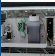
Nitrate module or ISE module for pH, conductivity & redox analysis (options)
