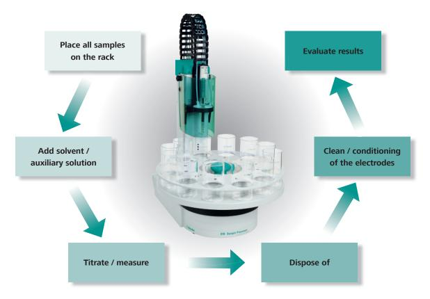
The 810 offers a wide choice of sample racks for different sample beakers. Depending on the sample size between 12 and 24 beakers can be processed in a series unattended.
