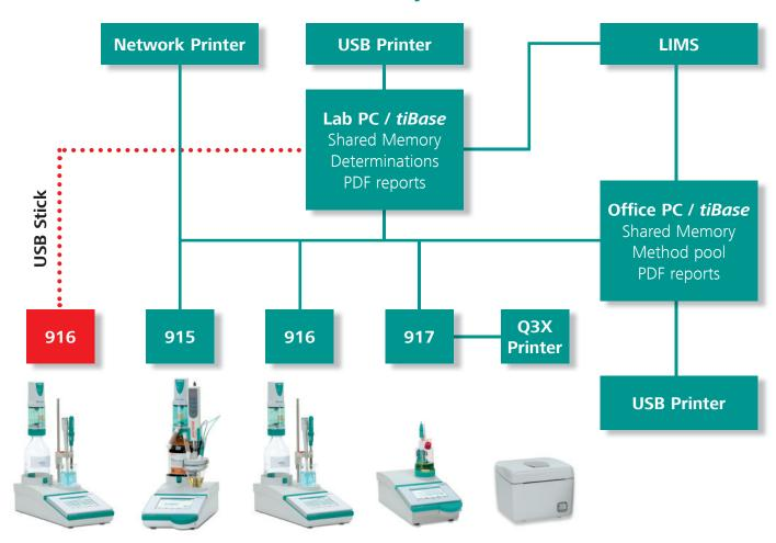
Integrate the Ti-Touch Family in your networked laboratory: automatically export PDF reports/determination files to your LIMS or into *tiBase* on your lab/office Computer, print on local or network printers, and share titration methods from a centralized network directory. Even data from instruments not connected to the network can be transferred via manual export to a USB memory stick.
